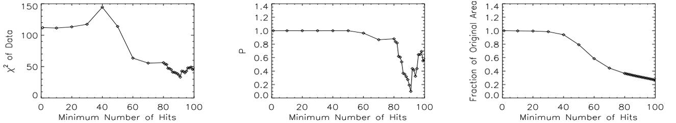
**Fig. 3.** From left to right,  $\chi^2$  statistic of the 143K03 noise map, its cumulative probability, and the fraction of available area for different values of the minimum number of hits at  $N_{side} = 128$ . This map becomes compatible with Gaussianity when the minimum number of hits is approximately 90.
